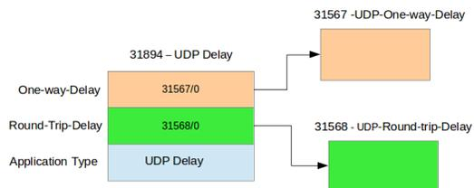
Figure 6. Example of a Composite Object: UDP-Delay
