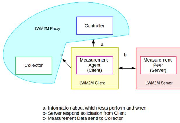
Figure 5. Functional schema of standardized measurement platform into LWM2M environment
