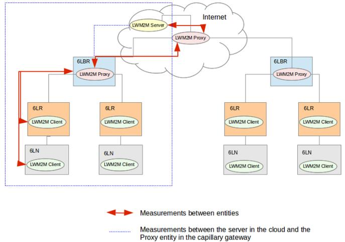
Figure 4. LWM2M Distributed Proxy Scenario in Capillary Networks
