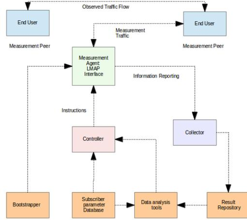
Figure 2. LMAP Measurement framework proposed
